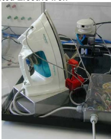
Figure 2: Instrumented remote access electric iron equipment at UWA
