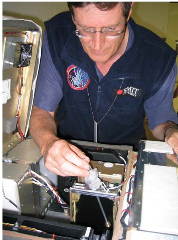
Figure 1: The payload locker showing the spider experiment habitat, Assoc Prof Lachlan Thompson demonstrates how the astronauts took web samples during the mission
