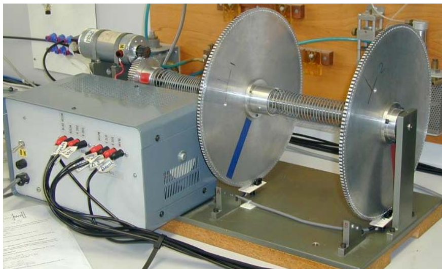
Figure 5: Torsion Vibration remote access equipment at UWA: an example where high rate real-time data needs to be shown to the user.
