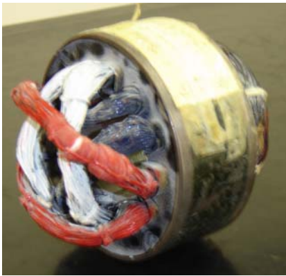
Fig.2: A two-pole stator
