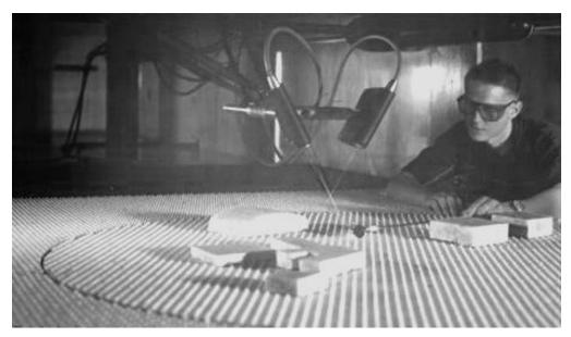
Figure 1. Officer Cadet David Nelson using laser Doppler velocimetry to measure runway turbulence generated by a model of nearby hangar and business park at Canberra Airport.
