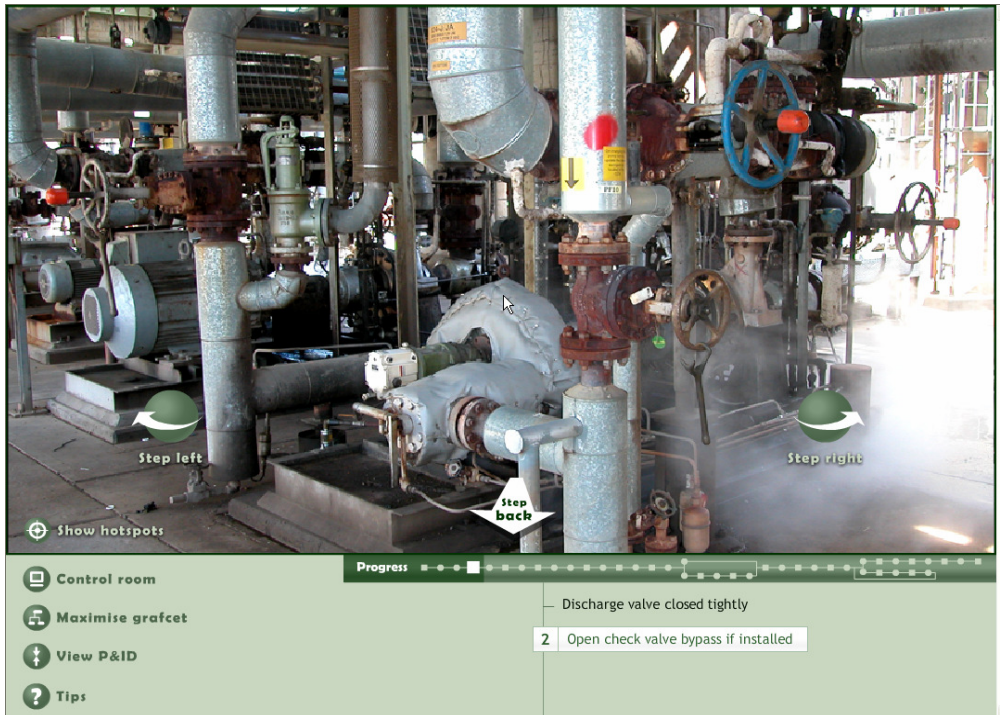
Figure 4 Pump isolation activity
