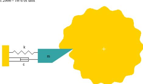
A lathe is found to chatter and its response is measured and found to be well modelled by a single degree of freedom system. You are required to stop chatter by the addition of a vibration absorber. You will be expected to work in teams of 3 or 4. Each team must have a member who can program and to that end only one double degree student with Maths or Computing can be in a team. If there is any difficulty in forming teams assistance will be provided.
