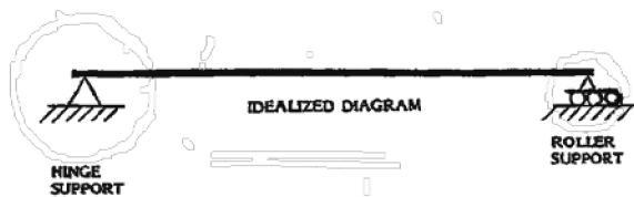
Figure 1: Simply supported beam
