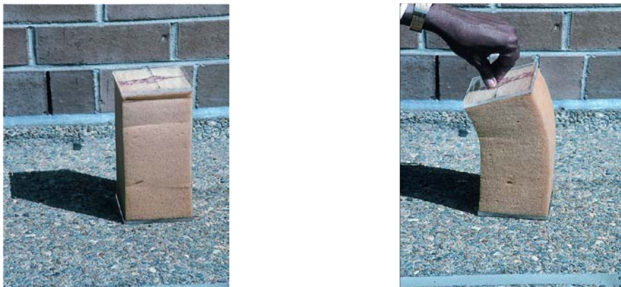
Figure 4: Eccentrically loaded member
