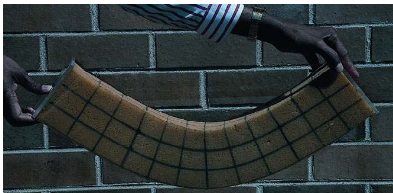
Figure 3: A plane section remains plane before and after bending
