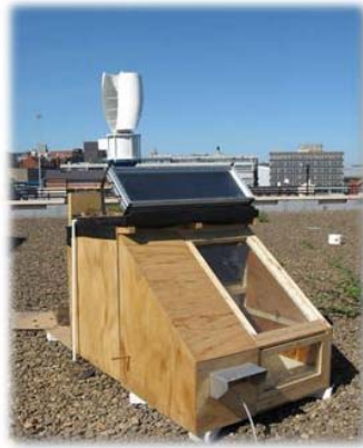
Figure 2 The one-fifth scale eco-house
