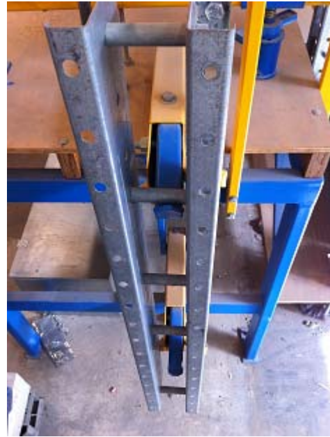
Figure 10: Detail of the climbing ratchet that a tutor will raise during the demonstration
