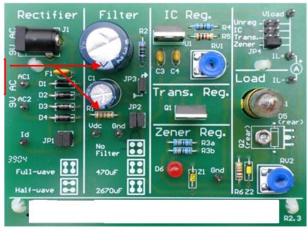
Figure 3 Fully Constructed Power Supply
