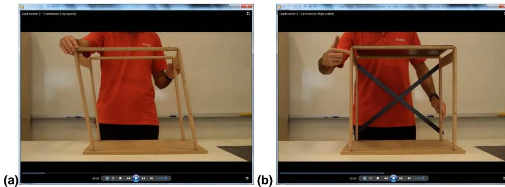
**Figure 3: Video demonstration of a 3D load transfer using a two-row structure: (a) no bracing, shear wall or slab (structure free to deform) and (b) bracing added at the back row and slab connecting the two rows together (stable structure)**
