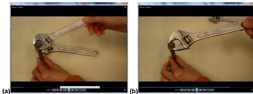
**Figure 1: Video demonstration of the concept of a moment using (a) a "short" and (b) a "long" lever arm**
