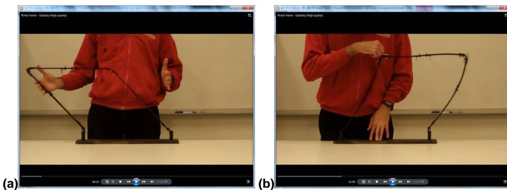
**Figure 4: Video demonstration of a frame with various restraint conditions and connection details: (a) hinged at the base and between beam and columns and (b) hinged at the base and fixed between beam and columns**
