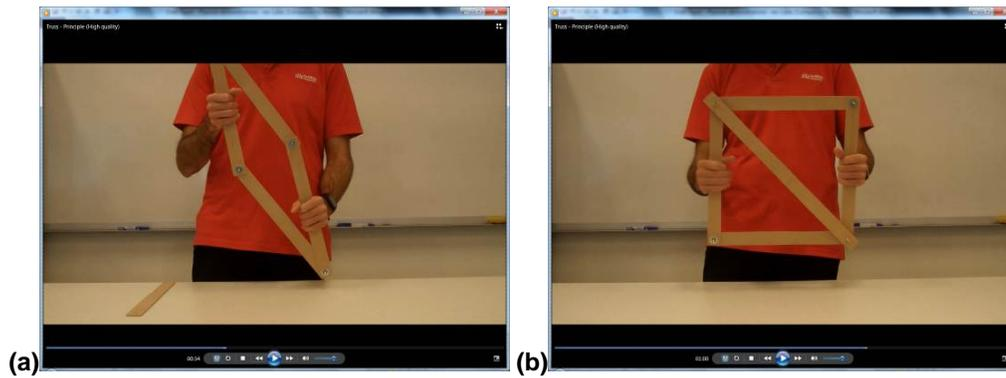
**Figure 2: Video demonstration of the principle of a truss (a) without (free to deform in shear) and (b) with diagonal bracing member**
