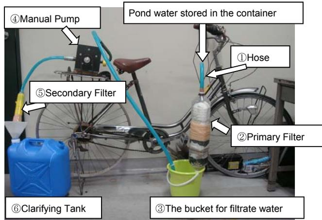
**Figure 9: Completed water-purification equipment**
