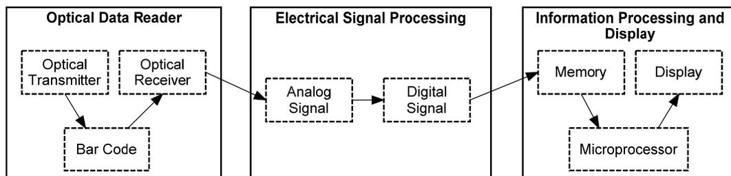
**Figure 1: Block diagram of generic barcode reader**
