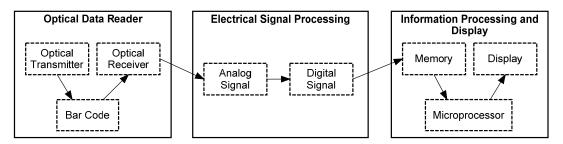
Figure 1: Block diagram of generic barcode reader
