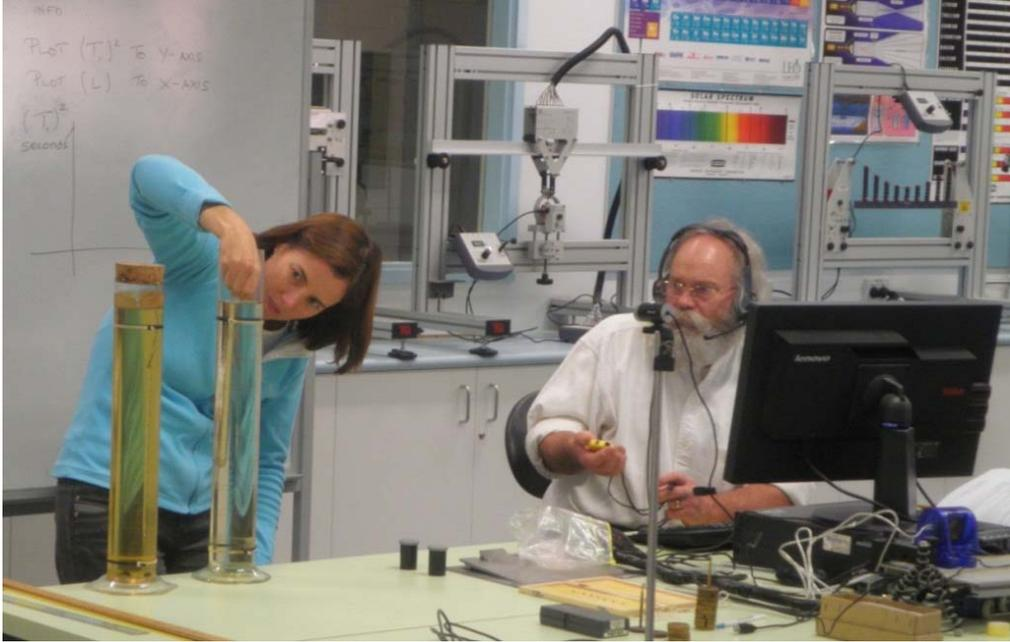
**Figure 3: Authors performing the fluid viscosity experiment via *E-live*. The first demonstrator is about to drop a small steel ball into a cylinder of glycerine. The second demonstrator measures the fall time with a stopwatch.**
