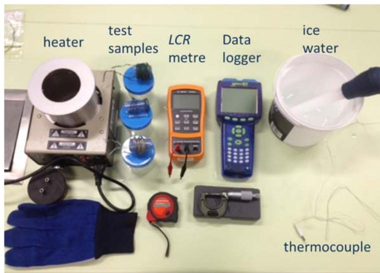
**Figure 1: Materials for the SEM111 practical on electrical resistivity of metal wires.**
