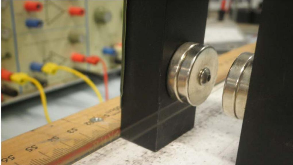
**Figure 6: Standing-waves practical. A wire vibrates as a sinusoidal current is passed between the poles of a magnet. The standing waves are difficult to see even in a still photograph.**
