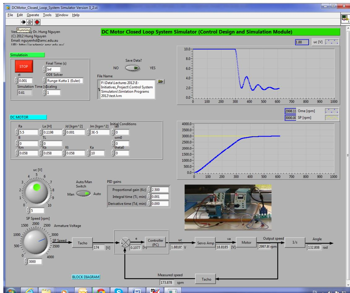
**Figure 4: DC motor control system simulator
