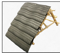
Figure 3. Final small-scale prototype roof
