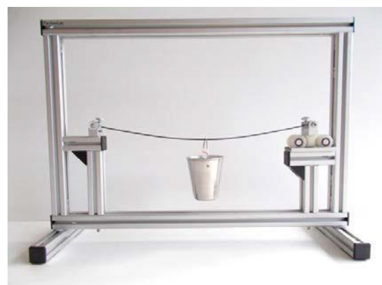
Figure 4: Simply supported CF beam central point load
