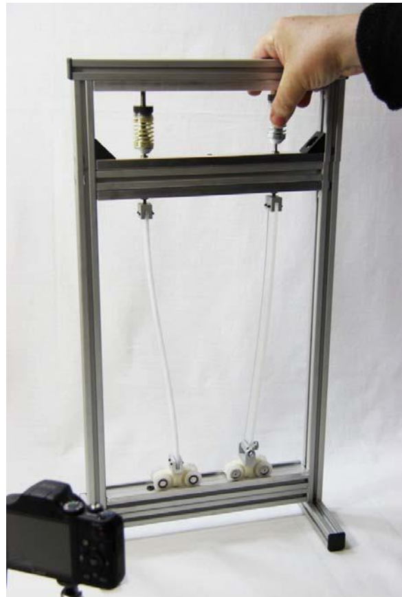
Figure 14: Column Buckling: Fixed-Pinned; Figure 15: Column Buckling: Fixed-Fixed Roller; Pinned-Pinned; Fixed-Fixed Fixed-Pinned Roller (Sway cases)
