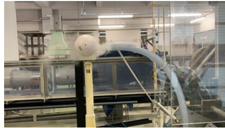
Figure 5: Visualized Magnus effect ( a\omega/U_\infty \approx 2 Re \approx 1.1 \times 10^4 )
