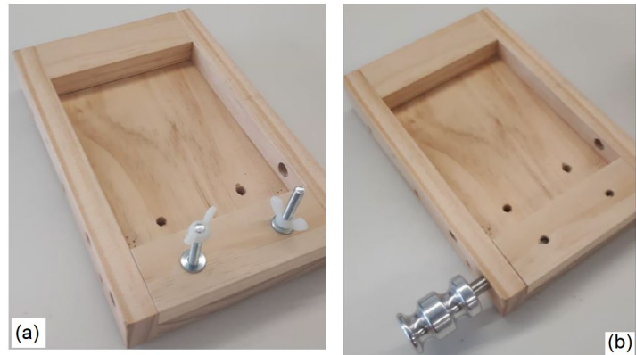
Figure 4: Illustrating SMED (a) non-SMED screw arrangement (b) SMED Screw arrangement
