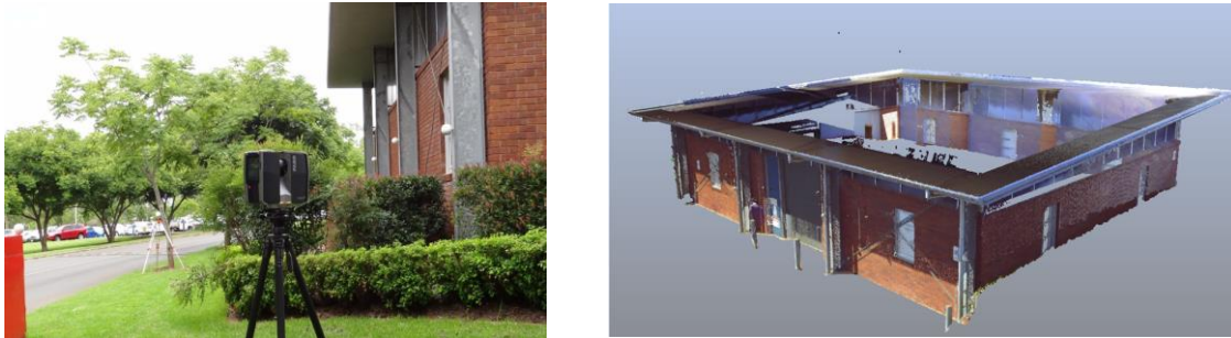
Figure 1: Field work in laser scanning and produced point cloud in TLS workshop
