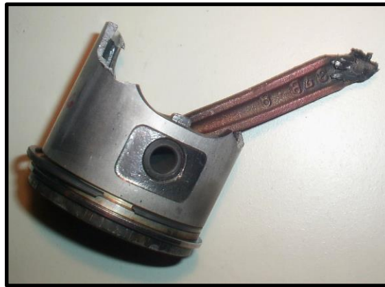
Figure 7.0 Picture of a broken piston and connecting rod from a scooter. DR Racing Parts 65 cc piston, standard Suzuki Katana AY50 connecting rod (Morini two-stroke engine).
