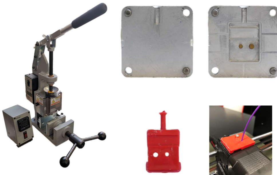
Figure 2: Injection moulder, mould, and LDPE moulded parts
