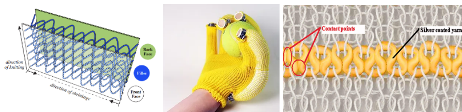
Figure 1: From left, spacer fabric (Albaugh et al., 2021), soft robotic glove (Luo et al., 2022), diagram of strain sensor (Atalay et al., 2016)
